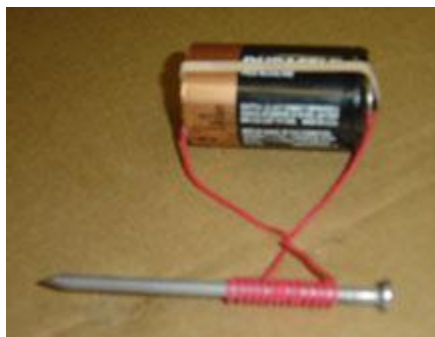
Figure 4. Set-up to make an electromagnet using a battery, wire and nail.
